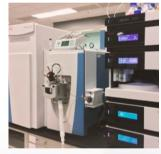
Thermo UPLC Q-Exactive HRMS instrument or equivalent
