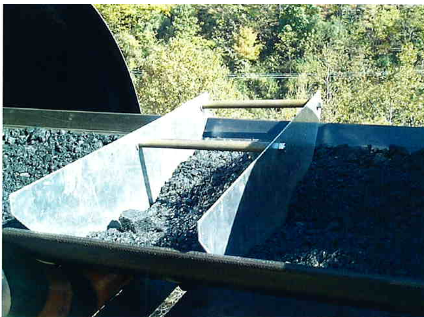
A minimum of 20 sets of stopped-belt reference samples and comparison samples are used to test for bias.
