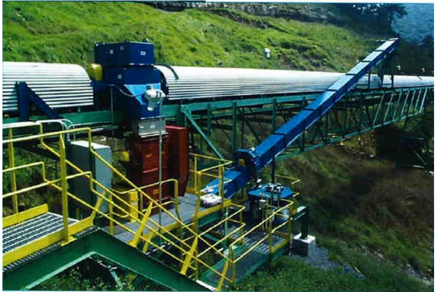
Mechanical sampling systems (MSSs) are used to sample bulk solids
